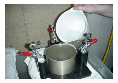
Fill the volumeter with water. The water level should be at or below the line drawn inside the volumeter. Approximately 0.375".
