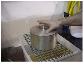
Place the lid on the volumeter and gently push down. Water should come slowly out of the post and sides of the lid. Rotate the lid on the volumeter to ensure good contact.
