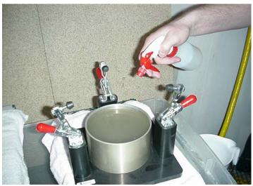
Spray the water surface with isopropyl (rubbing) alcohol to remove air bubbles.
