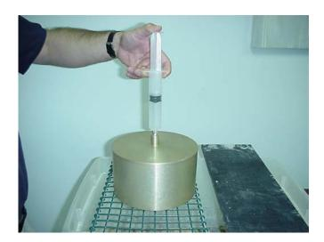
Position volumeter with the small hole to the front. Fill the volumeter with the syringe until water just comes out of the small hole. Insert needle completely to avoid introducing
