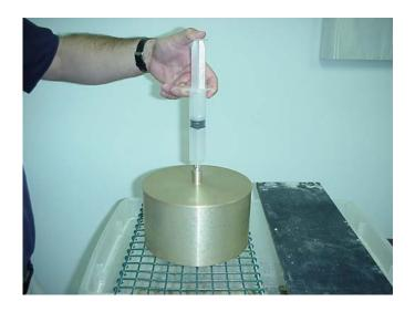
Position volumeter with the small hole to the front. Fill the volumeter with the syringe until water just comes out of the small hole. Insert needle completely to avoid introducing bubbles.
