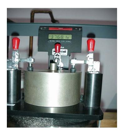
Weigh the container and the fixture. Don't worry about seepage around lid at this point. Record the weight.
