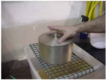
Fill the volumeter completely to the top with water and place the lid on making sure it is seated properly. Rotate the lid on the volumeter to ensure good contact.
