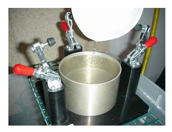
Place the fixture on a level surface!
