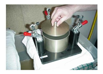
Place the lid on top of the volumeter. Make sure the 1/8" hole is facing the front.
