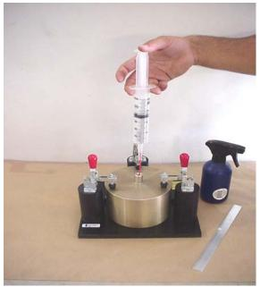
Using the syringe, gently fill the container with water through the center hole. Make certain the syringe tip is below the water surface in the volumeter. Stop as soon as water starts to come through the 0.125" hole on the lid
