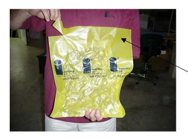
Cut one side approximately 3-4 inches. Spread both bags open and hold for 45 seconds, allowing the water to get in. When the water has filled the bag and the aggregate falls to the bottom cut the other side approximately 3-4 inches.
